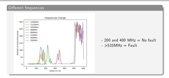
Possible to fault at different frequencies, by adapting the EM pulse delay.
