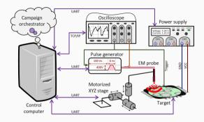
Set up for the realization of EM injection attack campaign
