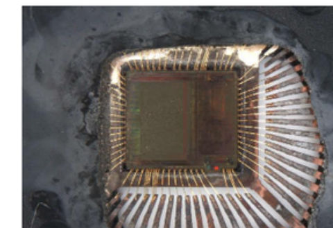
Backside of the chip with thinned silicon
